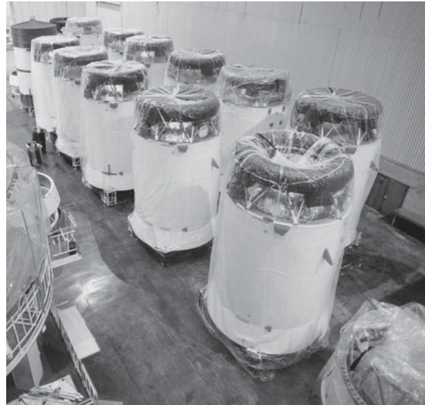
Fig. 3 A collection of Blok DM stages in their cylindrical aerodynamic casings, awaiting shipment from the RSC Energiya production facilities to Baikonur. The control units of the stages extend above the surrounding shrouds. (Copyright, International Launch Services.)
